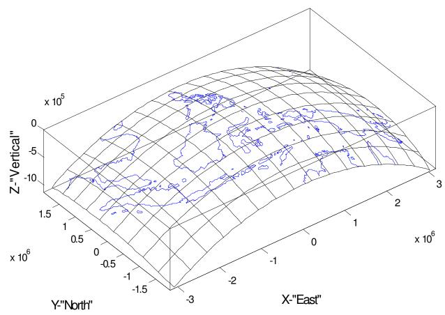
Indonesia in **ECEF-LH** as presented by Matlab. One can rotate this image in Matlab - or in a VE - to any perpendicular perspective, which will be free of distortion.
