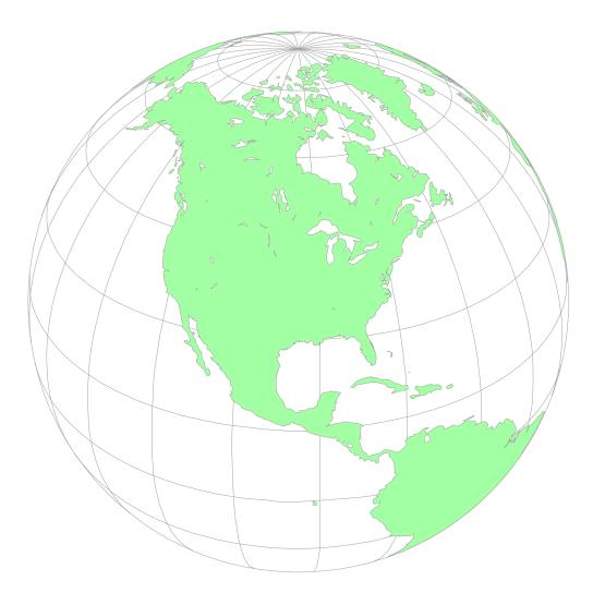
A graticule of curved parallels and curved meridians (latitudes and longitudes) intersect orthogonally on the ellipsoid. Height is measured along the normal, the straight line perpendicular to the ellipsoid surface.
