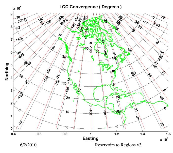
The red lines contour azimuth difference between grid and true north (i.e., convergence of the meridians) in degrees, varying (W to E) from -70° => 0° => +70°
