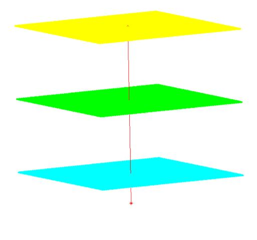
This cartoon of the reservoir off Ujung Pandang is in a G&G's typical VE perspective. It is 10km by 10km horizontally in plan view with three interpreted horizons: a yellow sealevel surface, basement 10km deep in blue and one in between in green. A well is drilled through basement.
