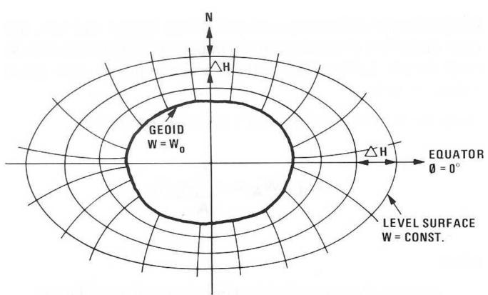
Elevation is measured along the (slightly curved) vertical, which is perpendicular to the irregularly layered geopotential surfaces of the earth. The geopotential surface at mean sea level is called the geoid. (Graphic from Hoar, 1982.)
